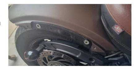
Place rack over the top of rear fender and attach to the threaded holes on the sides of the rear fender with the M8 x 20mm Flange bolt provided with the rack. (Blue Thread Locker is recommended at this point)
