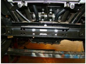
Install winch to winch plate with hardware provided with winch. Now place mount in place on top of support plate and bolt down with  $5/16 \times 1$  hex bolts and 4-flat washers and nylock nuts, secure in back with  $3/8 \times 1$  hex bolts washers and nylock nuts.
