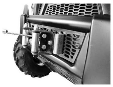
Use the roller fairlead brackets if installing a standard size fairlead or hawse.
