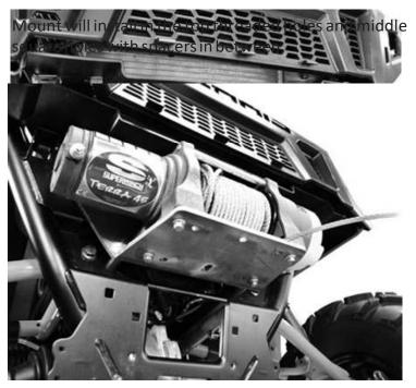
Bolt the winch in place using the hardware provided with your winch.
