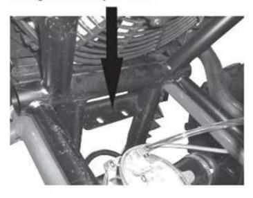
Carriage bolts install from the top of the bumper bracket. Roller fairlead bracket and front of mount install below the bumper bracket.
