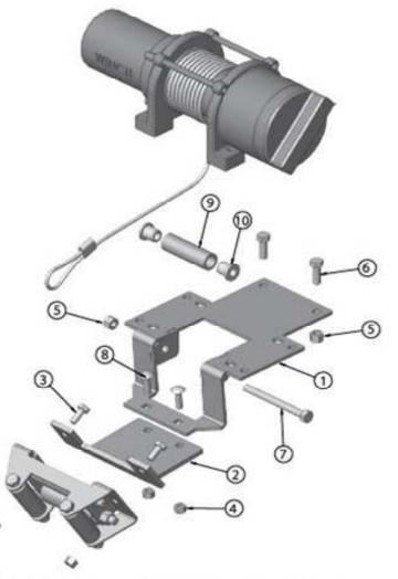
Back of the mount plate bolts on top of this frame bracket.
