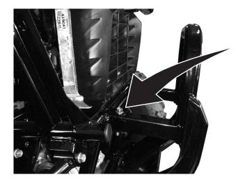
Put the bumper with winch and mount back on the machine. Install the factory bolts back in place through the bumper and back of the winch mount.
