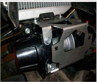
After winch and mount are secure you can re-attach the Plastic frill under the headlights with the 10 plastic pop in plugs.
