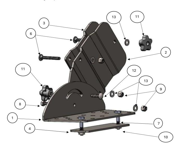
First page shows the mounting bracket which can be used to mount to solid services and some tube type racks by sandwiching between the base plate (item 1) and the mounting plate (item 4). The mounting plate can be moved around and attached to the base plate in many locations.
